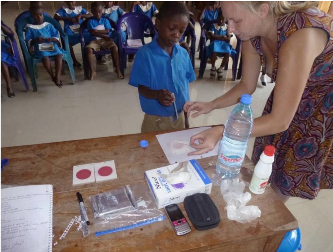
In Cary's water sanitation class a student uses 3M Petrifilm to test for coliform and E. coli.
